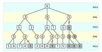
**Figure 2:** An illustration of alpha-beta pruning. The grayed-out subtrees need not be explored (when moves are evaluated from left to right), since we know the group of subtress as a whole yields the value of an equivalent subtree or worse, and as such cannot influence the final result. The max and min levels represent the turn of the player and the adversary, respectively.
